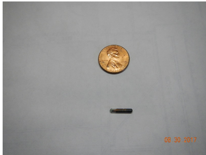
A PIT tag (glass encapsulated transponder)
